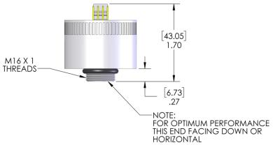
(1) In air @ 25° C and 1 atm. Expected life varies inversely with changes in O2 concentration, temperature, pressure. PPM Sensors Expected life based on < 1000 PPM
